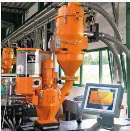
G-mixer with two Kō dosing stations and the new SLT and MCT control units with 7" colour touch display
