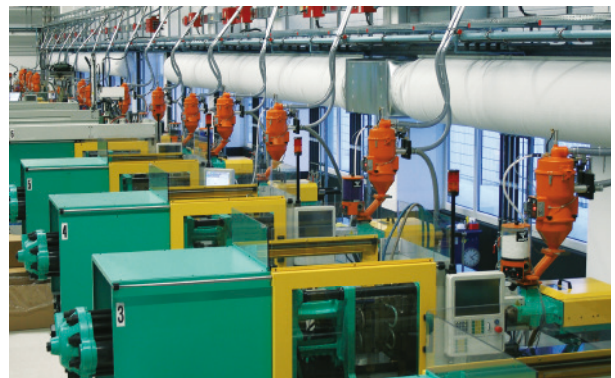
Central material supply system with direct colouring Exemplary system for flexible material supply with Industry 4.0
