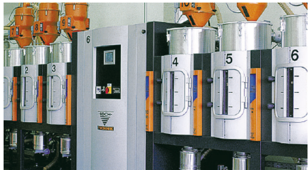
EKO 300 with 6 x 100 litre drying containers
