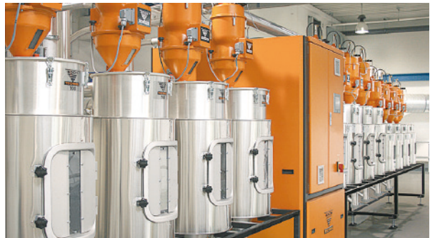
CKT 500 granule dryer with 12 drying containers
